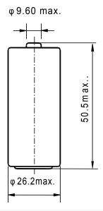
Size unit:mm (GB1804-m if tolerance is not specified)
